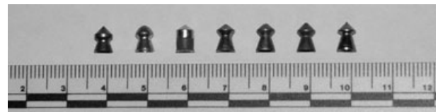
FIG. 11—Photograph of pointed pellets in Group II-P. Pellets listed from left to right include: Crosman Super Point, Daily Lead Free, Skenco Hyper-Velocity Type II (blue sabot), Qiang Yuan, Diabolo BOXER, JSB Straton Diabolo Fur Luftwaffen (Seam on side), and RWS Superpoint Extra.
