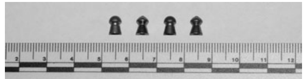
FIG. 3—Photograph of domed pellets in Group III-D. Pellets listed from left to right include: Crosman Ultra Magnum, Beeman Kodiak Match Extra Heavy, Crosman Copperhead (Bubble Pack), and Beeman Kodiak Extra Heavy.
