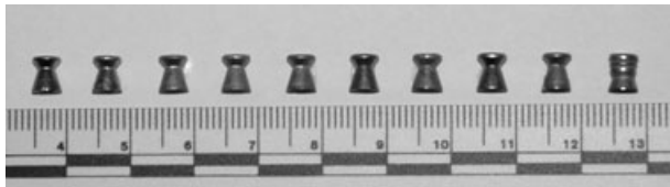
FIG. 6—Photograph of wadcutter pellets in Group II-W. Pellets listed from left to right include: RWS Meisterkugeln, RWS Dynamil Nobel, JSB Match Diabolo Fur Luftpistolen, Diabolo Match “R,” JSB Match Diabolo S100 Fur Luftpistolen, Beeman Laser Sport (Sampler), Diabolo LUX, RWS-DynamilNobel, JSB Fur Luftpistolen, Luftpistolen, Luftpistolen and Beeman Silver Ace (Sampler) (3 ring head).
