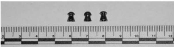
FIG. 14—Photograph of hollow point pellets in Group I-HP. Pellets listed from left to right include: Beeman Silver Bear (Sampler), Crosman Hunting Pellet, and RWS Super - H - Point.
